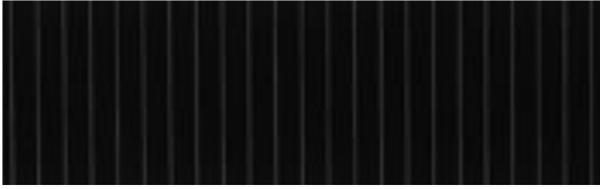
Fig. 1. Photograph of a gridline TLM pattern, as cut from a solar cell. Sample width is 10 mm and length is 35 mm.
